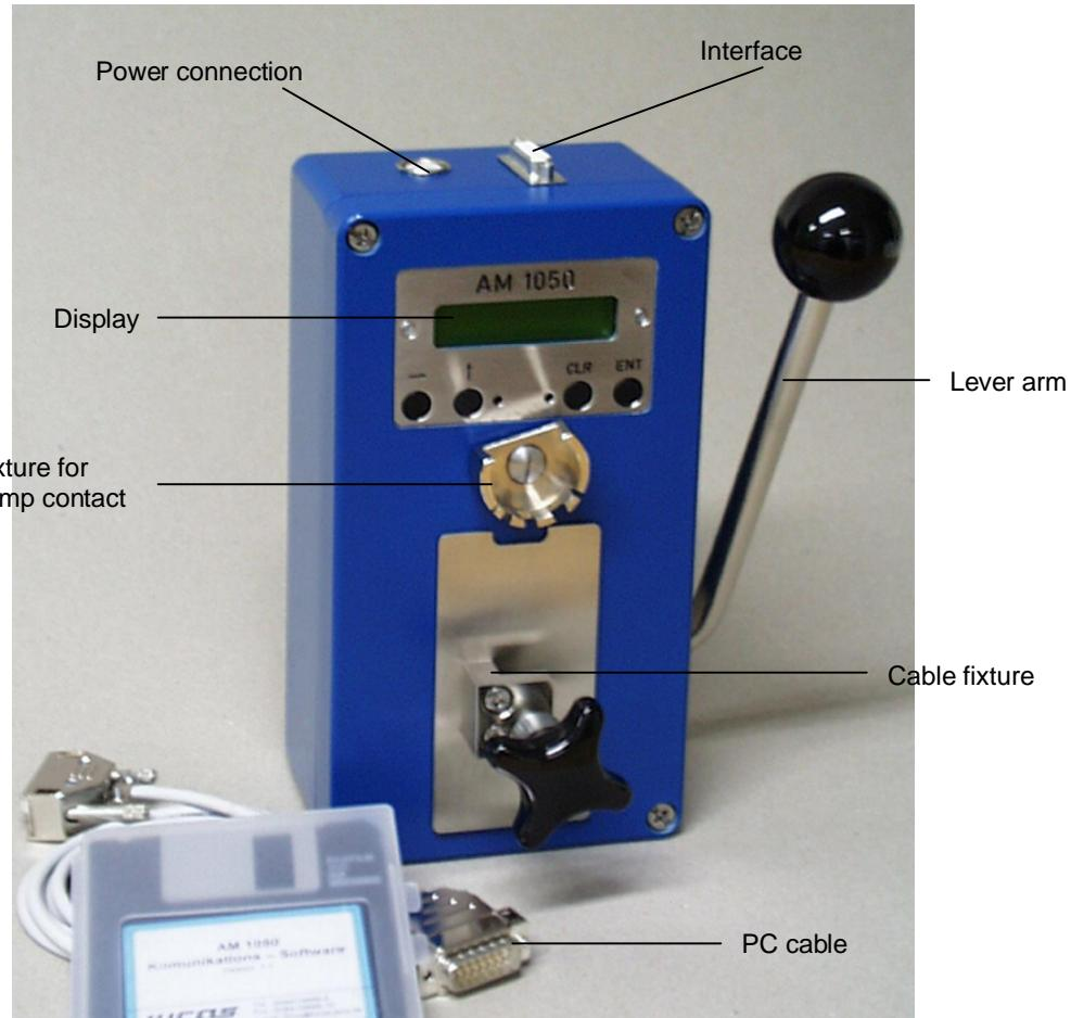
The digital Stripping Force Tester AM 1050 is a compact and easy to handle testing device. It is used to measure the pull apart force for crimped connectors and therefore to assure the quality in cable manufacturing.
